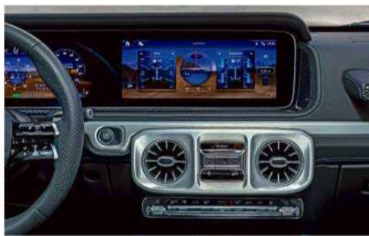
INFOTAINMENT 'Off-road cockpit' displays data such as an artificial horizon, a compass, plus altitude, steering angle, tyre pressures and torque loads
